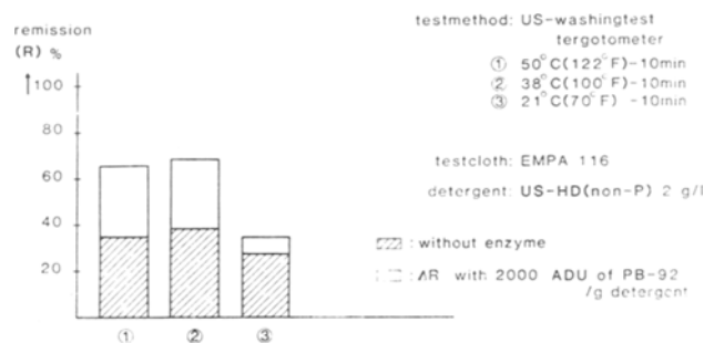
FIG. 4. The effect of the washing temperature on the cleaning result (PB-92).
